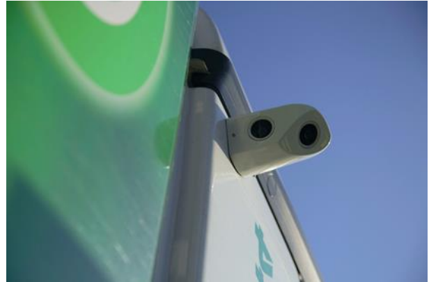
The intelligent rear-view mirror provides data in real time, Copyright AVI Systems
